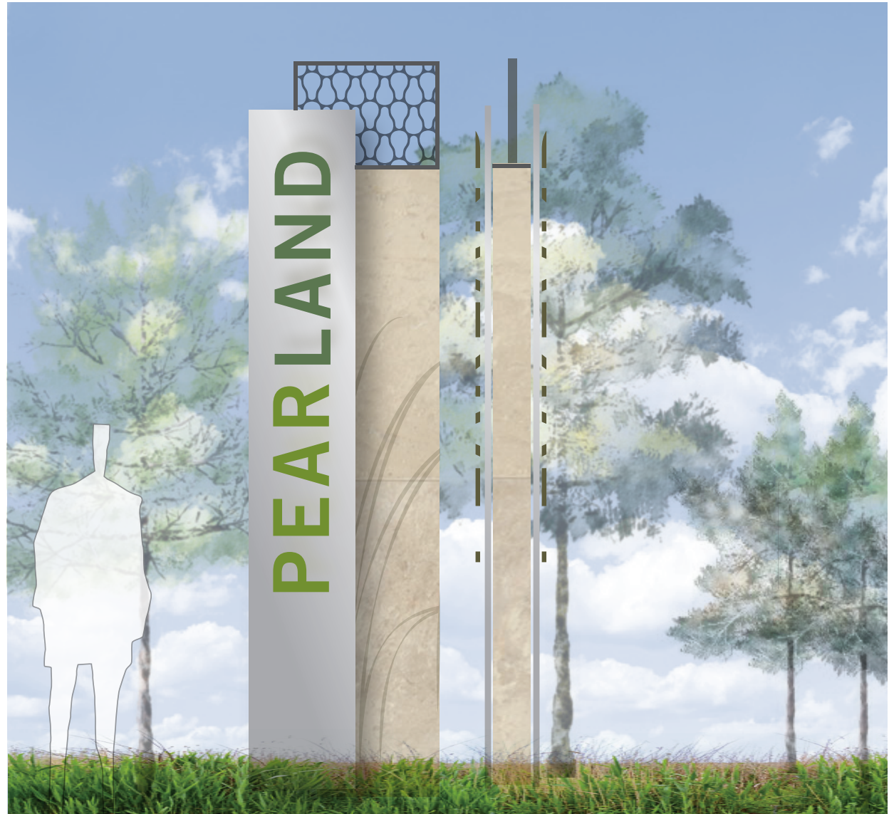
Fig 2.1 Graphic representation of Pearland Gateway signage. Overall height of sign is roughly 14'-0"
