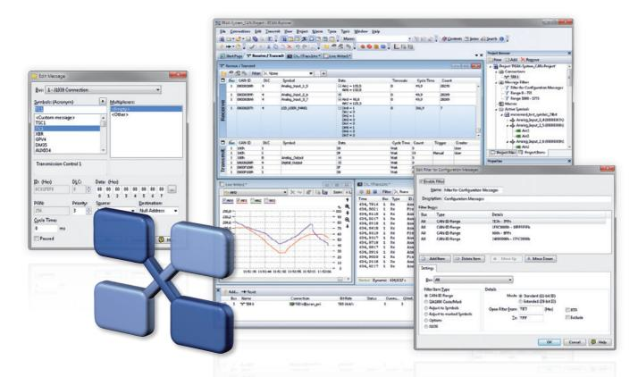
PCAN-Explorer is a universal tool for monitoring data traffic on a CAN network. For easy and clear allocation of the individual messages, these can be identified as so-called symbols. The integrated VBScript support allows the creation of macros to automate complex tasks. The integrated data logger means that the data traffic of a bus can be recorded, analyzed, and stored. PCAN-Explorer is designed as automation server and can therefore be remote controlled through scripts.
