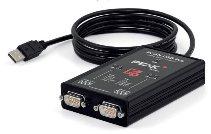
The PCAN-USB Pro FD adapter enables the connection of CAN FD and LIN networks to a computer via USB. Two field busses can be connected at the same time, up to four with appropriate adapter cables (2 x CAN FD, 2 x LIN). Each CAN FD channel is separately isolated against USB and LIN with a maximum of 500 Volts. Its robust aluminum casing makes the PCAN-USB Pro FD adapter suitable for mobile applications.
