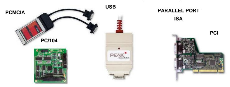
**PCAN** interfaces support both 11 bit ID and 29 bit ID CAN specifications with a maximum speed of 1Mbaud. They use the SJA1000 CAN-controller and the 82C251 driver. The CAN-bus connection is via a 9-pin SUB-D plug, whose pin assignments conform to the CiA recommendation. No termination is included in the interfaces. Optoisolated versions are available if required and most interfaces can be supplied with one or two ports.
