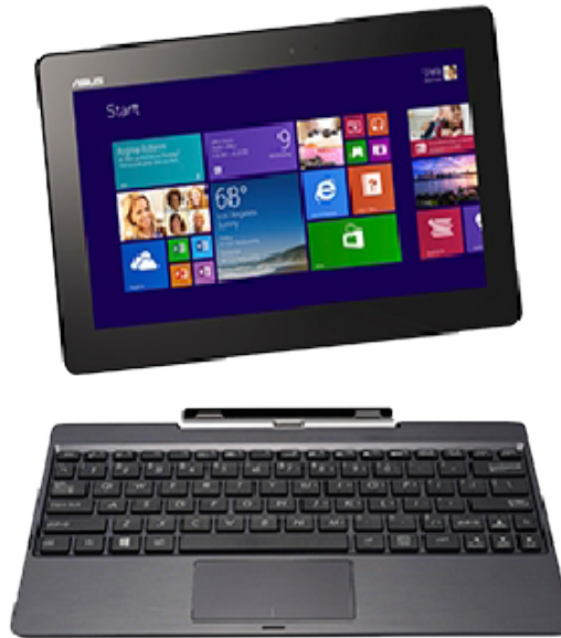
Hybrid or "2 in 1" computer (a mobile device that has the features of a tablet and a laptop, such as a touch screen and a keyboard)
