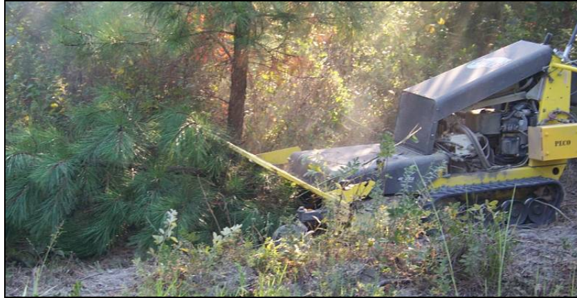
Figure 17: Cutting Heads Engaging Tree After Being Pushed by Safety Bar
