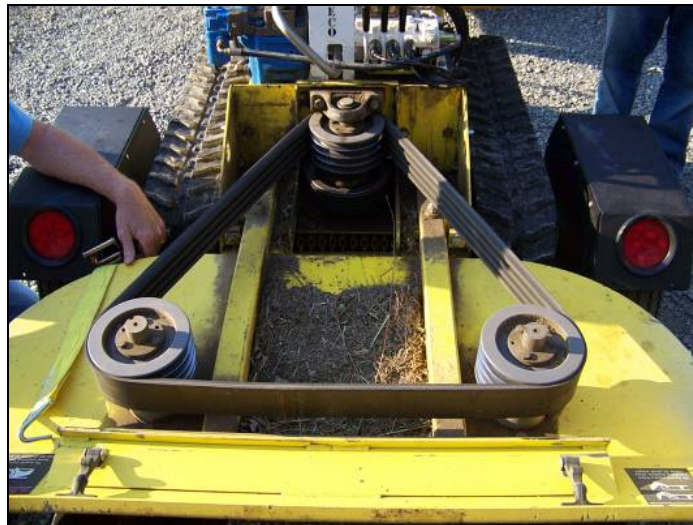
Figure 28: Cutting Blade Belt (Top Cover Removed for This Photo)
