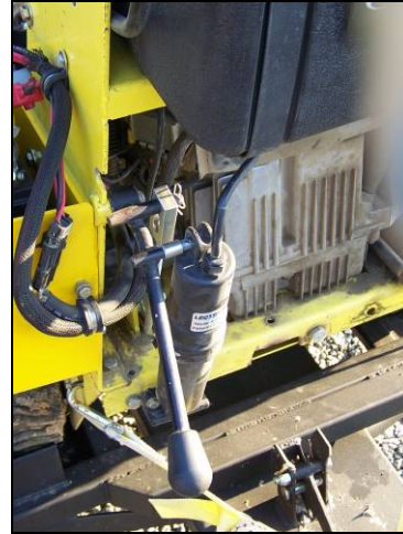
Figure 9: Cutter Engaging Lever After Modifications (Hydraulic Addition allows Operator Push-button Cutter Engagement)
