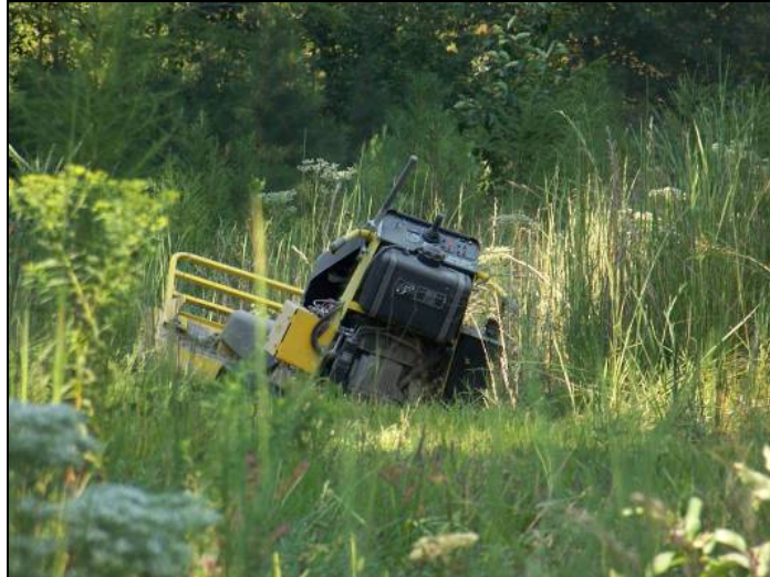
Figure 20: Peco Cutter Encountering 26.7 cm Deep Gully at Test Site B
