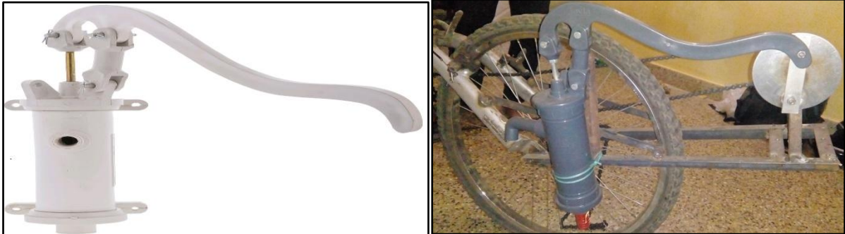
Fig. 5 assembly of reciprocating pump on bicycle
