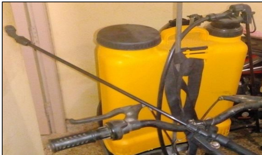
Fig. 4 position of pedal operated agro sprayer on bicycle
