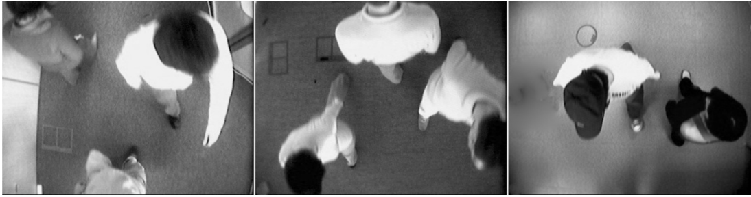
Figure 1.4: Video recorded from an overhead camera.[BMB08]. Such scenes present considerably less difficulty, due to the uniform size of people as seen from above, and almost no occlusion.
