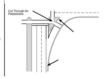
**Refuge Islands:** Where refuge islands are included, the tip of the island should extend through the crosswalk, with a curb cut for accessibility. Refuge islands should be clear of obstructions and have adequate drainage. They should be at least 12 feet long or the width of the crosswalk (whichever is greater) and 60 feet square. Recommended refuge island widths are as follows:
