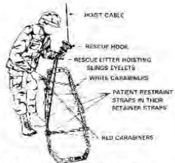
HOOKING THE STOKES LITTER TO THE RESCUE HOIST
