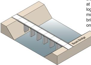
Beam bridges consist of horizontal beams that are supported at each end by piers. The earliest beam bridges were simple logs that sat across streams and other simple structures. In modern times, beam bridges include large-box steel girder bridges. The weight on top of the beam pushes straight down on the piers at either end of the bridge.
