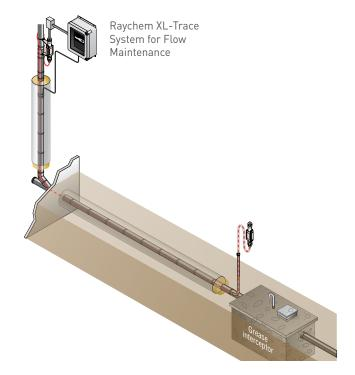
The energy-efficient XL-Trace heating cable keeps total operating costs down by adjusting power output in response to ambient temperatures. Easy to install, the XL-Trace cable can be cut to length on site and overlapped at valves, flanges, and pumps.
