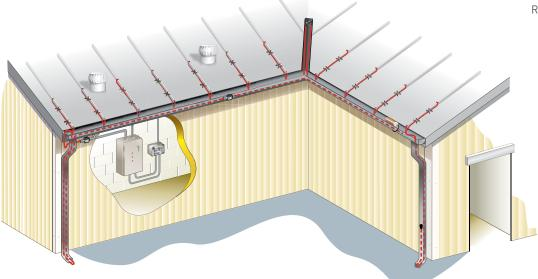
Raychem IceStop System for Roof & Gutter De-Icing
