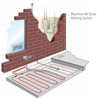
The Raychem ElectroMelt system incorporates a rugged cut-to-length self-regulating heating cable that automatically adjusts power output in response to concrete temperature.
