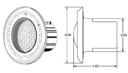
Note: All 120 volt pool and spa lights must be connected to a branch circuit protected by a ground fault circuit interrupter (GFCI).
