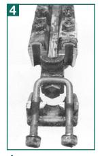
**4** Flourocarbon and Moly DiSulfide coatings too easliy penetrated
