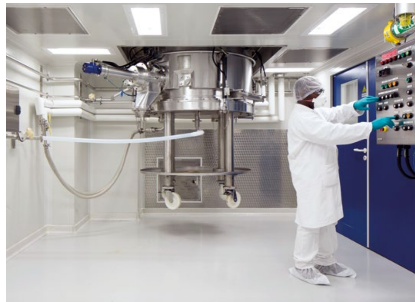
Drying of the final crude API in a filter dryer at CordenPharma Brussels (BE).
