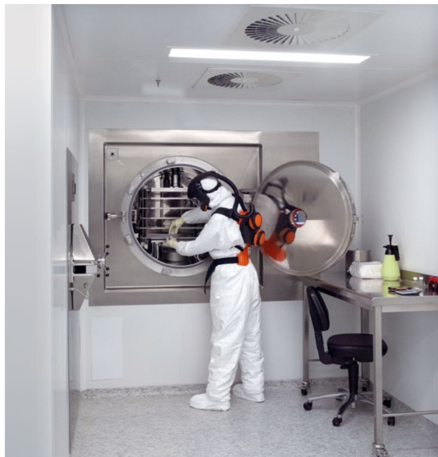
Sampling of a final API to support homogeneity testing plan at CordenPharma Switzerland.
