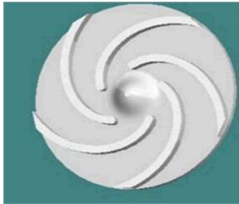
Gambar 2.6 Impeller Semi-terbuka Sumber : www.engineersedge.com
