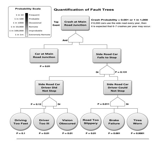
Figure 7.4 Fault Tree Analysis of the Possible Causes of a Crash at the Main Road Junction
