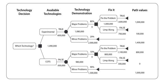
Figure 7.2: Example of Decision Tree for Choosing between an Experimental Technology vs. Commercial Off the Sheet (COTS) Technology.
