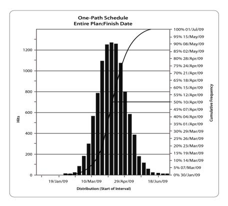
Figure 7.5: Example Histogram from Monte Carlo Simulation of a Project Schedule Source: Pertmaster v 8.0 Primavera Pertmaster
