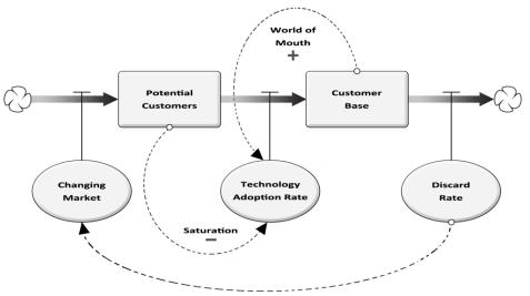
Figure 7.7 Example of a Simple System Dynamics Model with Feedback Loops
