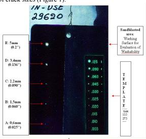
Figure 1 Initial system capability test of a calibrated test panel PSM-5 upon receipt. Penetrant Type I (fluorescent), Method D, sensitivity Level 4 (ultra-high), form a (dry developer)
