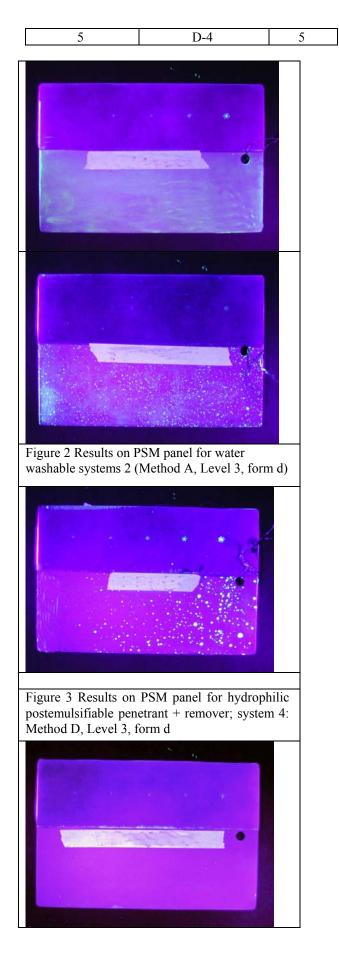
Figure 4 Results on PSM panel for lipophilic postemulsifiable penetrant + emulsifier; system 3: Method B, Level 3, form d
