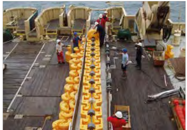
Polyspace installation on offshore vessel
