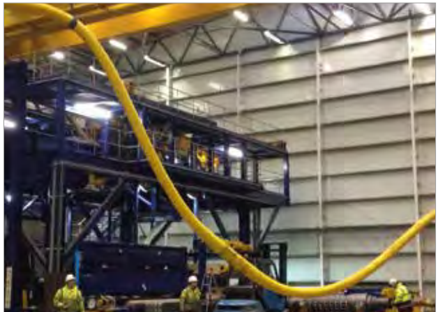
Full-scale testing of Trelleborg's NjordGuard™ integrated protection system
