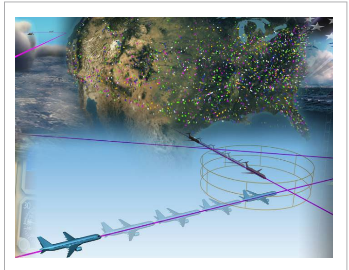
Figure 15 – Trajectory Based Operations describe an environment where traffic is managed based on where aircraft are and where they will be located as they progress along their respective flight paths.
