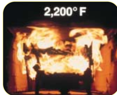
UL 910 Tunnel Test Apparatus
