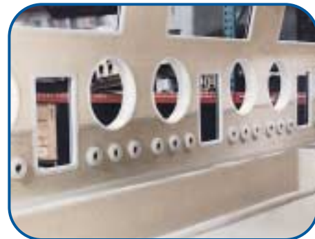
Chemical Handling Systems KYNAR® PVDF glove box constructed to resist a combination of radioactivity and acids.
