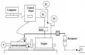
Fig. 3 : Experimental set up of engine Procedure
