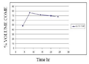
Fig. 2.3 : Effect of Reaction Time on Bio-Diesel Production (CH<sub>2</sub>OH=20%KOH=0.5%, Reaction Temperature 60°c).
