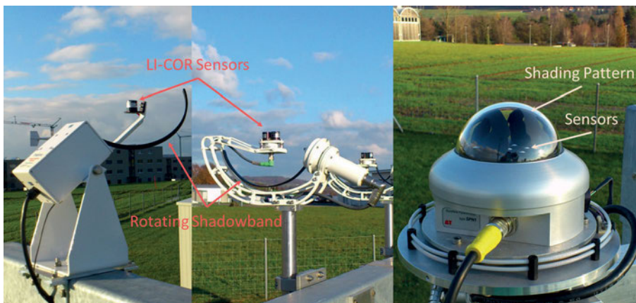
Figure 1: Rotating Shadowband Irradiometers (left: CSPA; center: CSPB) and SPN1 Shading Pattern Pyranometer (right).
