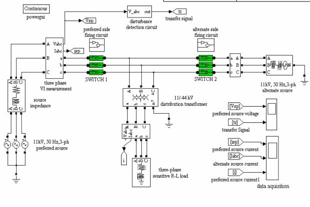
Fig.5: Simulink model of three-phase STS system
