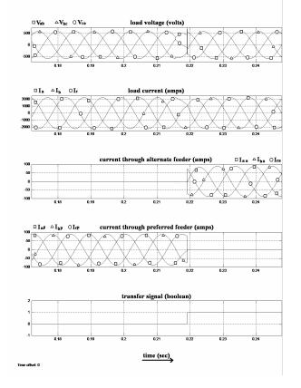
Fig.14: Load current and transfer signal
