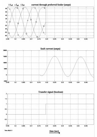
Fig.15: Fault current and transfer signal ISSN: 1991-8763
