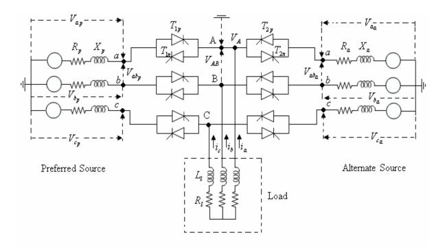
Fig.12 : IEEE STS - I system configured with RL load
