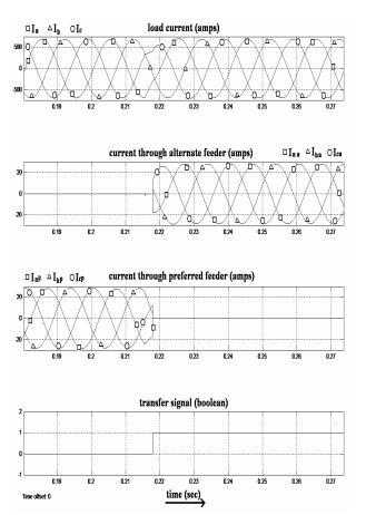
Fig.7: Current through load
