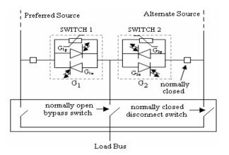
Fig.1: Basic structure of a single-phase STS
