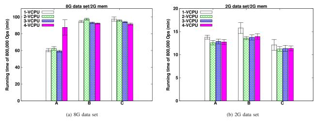
Figure 3: Average running time of 800,000 operations for three pre-defined YCSB workloads in virtualized environments. Error bars represent 95% confidence intervals.
