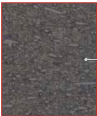
PA 6.6T + Solid Lubricant + Fillers
