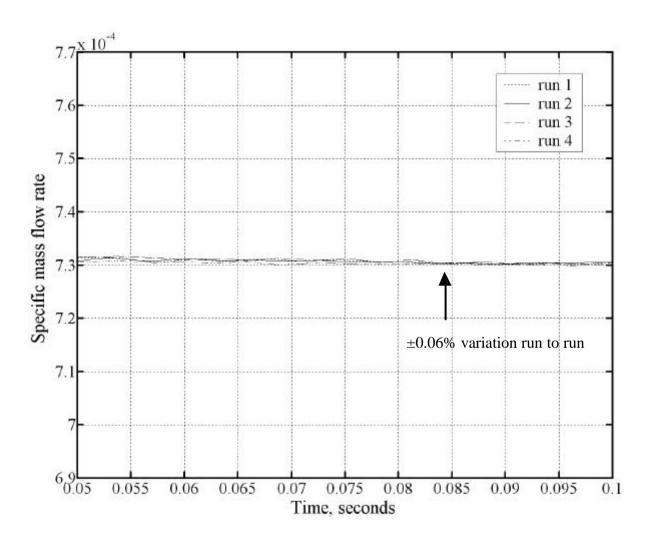
Q263 Through flow results, mass flow = 29.2 kg, specific mass flow =7.2x10<sup>-4</sup> Department of Engineering Science
