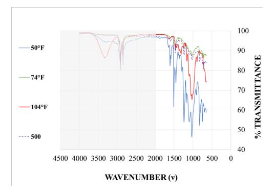
Figure 6.8: Material 2 FTIR results with varying cure temperature
