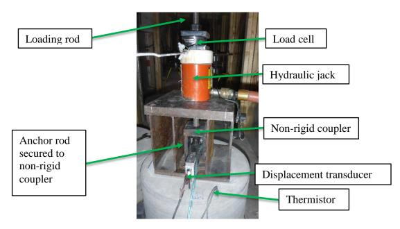
**Figure 4.12: Short-term test apparatus**
