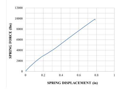
**Figure 4.16: Example of spring calibration**
