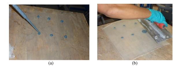
Figure 6.1: (a) Delivery of adhesive onto nonstick wax paper; (b) use of steel finishing trowel to prepare disk
