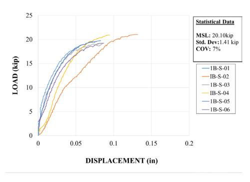
Figure 5.2: Material 1B short-term tests: load vs. displacement
