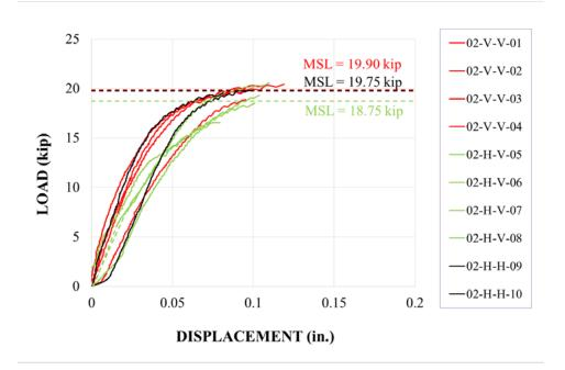
Figure 5.19: Material 2 installation direction: load vs. displacement
