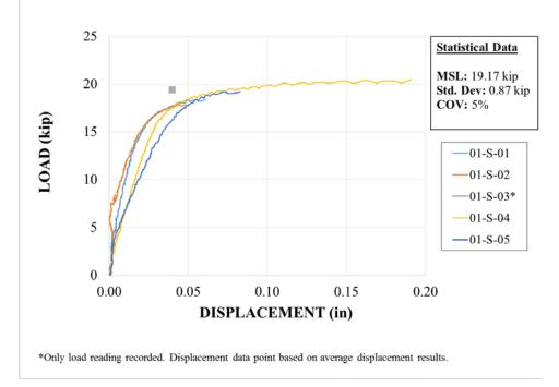
Figure 5.1: Material 1 short-term tests: load vs. displacement
