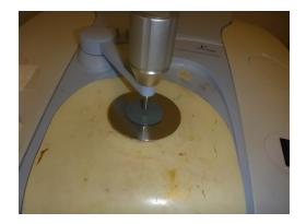
Figure 6.4: FTIR test of epoxy sample
