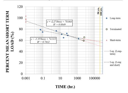
Figure 5.16: Material 1: Short-term tests plotted at time zero
