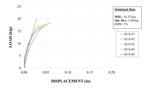
Figure 5.3: Material 2 short-term tests: load vs. displacement
