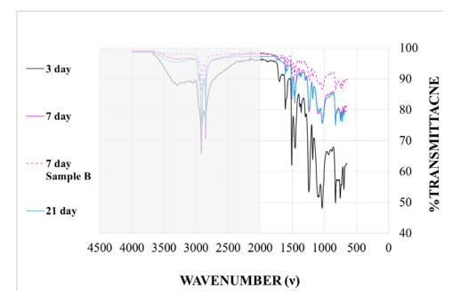
Figure 6.15: Material 3 FTIR results with varying cure time
