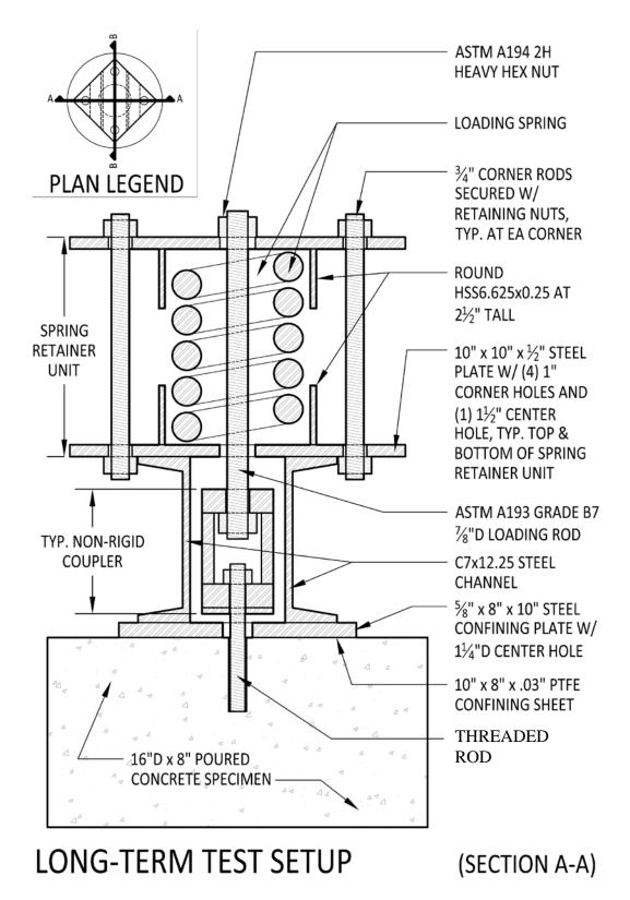
Figure 4.17: Long-term test apparatus, Section A-A
