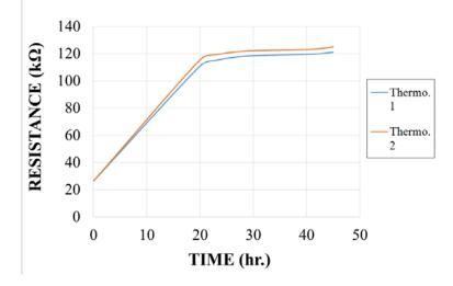
Figure 4.2: Resistance vs. time plot of sample concrete block
