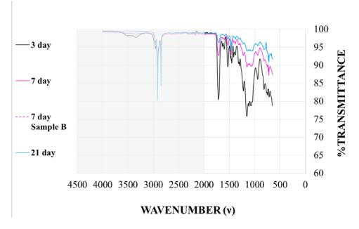
Figure 6.17: Material 7 FTIR results with varying cure time
