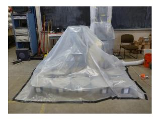
Figure 4.4: Conditioning of specimens prior to drilling
