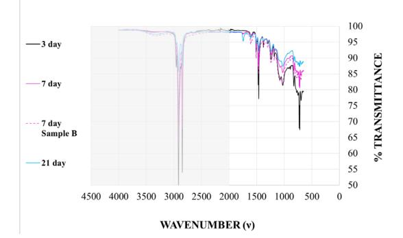
Figure 6.12: Material 1 FTIR results with varying cure time
