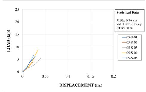
Figure 5.7: Material 5 short-term tests: load vs. displacement
