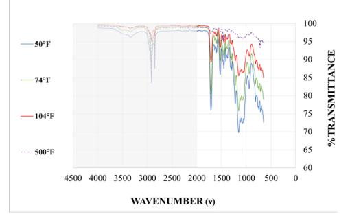
Figure 6.11: Material 7 FTIR results with varying cure temperature
