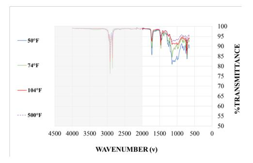
Figure 6.10: Material 4 FTIR results with varying cure temperature
