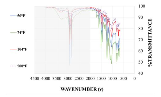
Figure 6.9: Material 3 FTIR results with varying cure temperature
