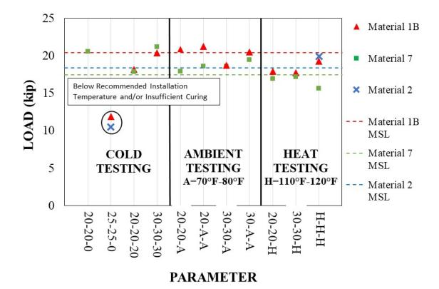
Figure 5.21: Summary of extreme in-service temperature test results
