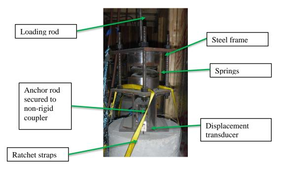
Figure 4.15: Long-term test apparatus
