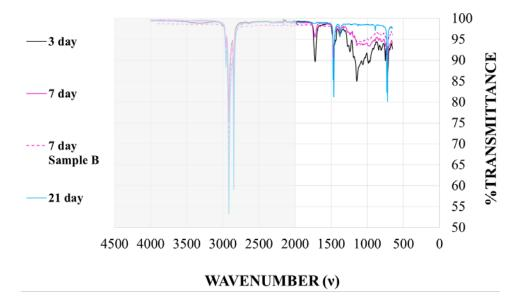
Figure 6.16: Material 4 FTIR results with varying cure time
