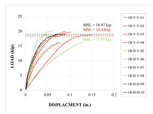
Figure 5.18: Material 1B installation direction: load vs. displacement
