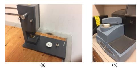
Figure 6.5: (a) Preparation of sample for DSC testing; (b) DSC testing instrument
