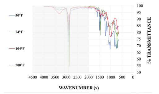
Figure 6.6: Material 1 FTIR results with varying cure temperature
