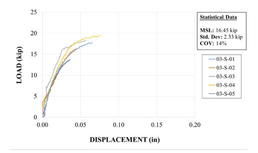
Figure 5.4: Material 3 short-term tests: load vs. displacement
