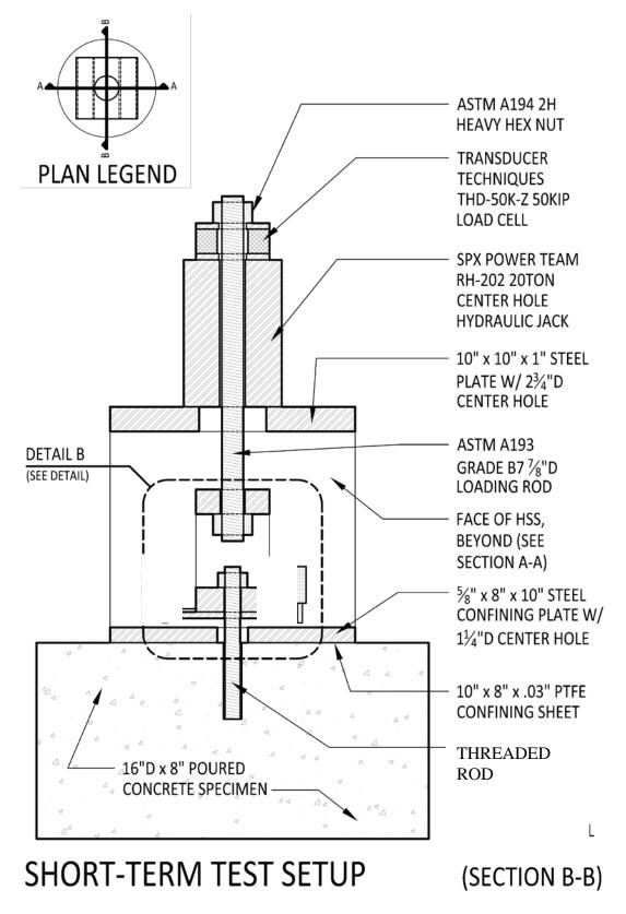
Figure 4.14: Short-term apparatus, Section B-B
