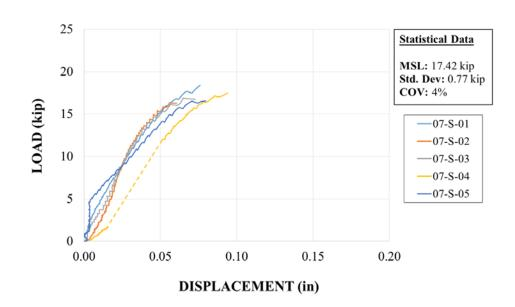
Figure 5.9: Material 7 short-term tests: load vs. displacement
