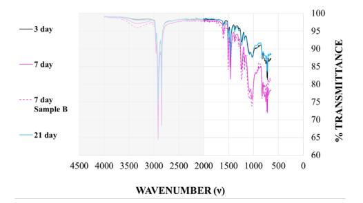
Figure 6.13: Material 1B FTIR results with varying cure time
