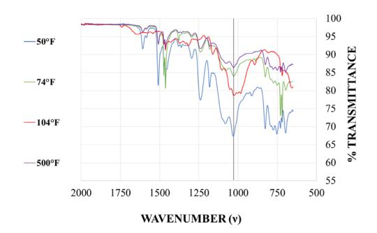
Figure 6.25: Normalized Material 1 FTIR results with varying cure temperatures
