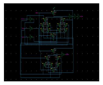
Figure 4. Dual rail adder
