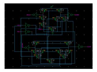
Figure 5. Dual rail logic
