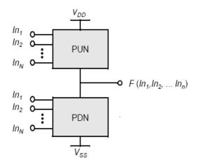
Figure 1. Static cmos logic
