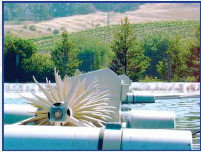
These vineyard aerators use a duplex coating of hot-dip galvanizing and paint to protect against tropical sea water and salt spray exposure.
