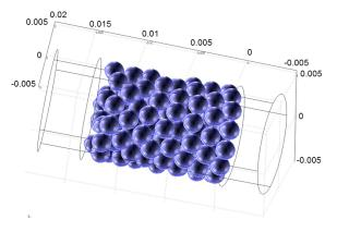
Fig. 1 Irregular packing of 150 spherical beads in a cylindrical tube
