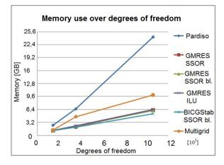
Fig. 3 Memory usage over degrees of freedom for different linear solvers and preconditioners
