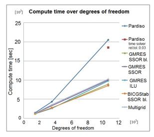
Fig. 2 Compute time over degrees of freedom for different linear solvers and preconditioners
