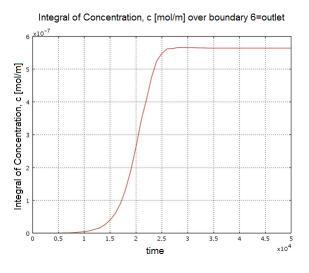
Fig. 4 Integral of outlet concentration over column cross section as function of time
