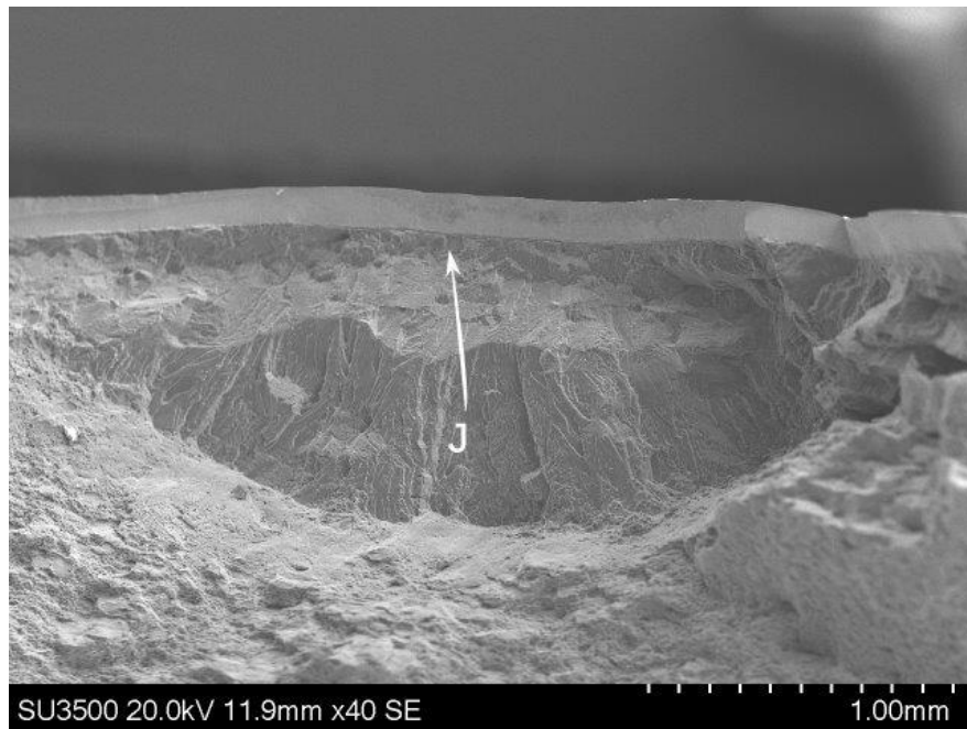
Figure 4.46: Location J on fracture surface of Specimen H13, which corresponds to the support side of the impact indentation.
