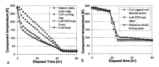
**FIGURE 2.** Temperature vs. time traces during the initial cool-down of the L-coil and cryostat. a) for components cooled by the cryocooler. b) for components cooled by the liquid nitrogen reservoir.
