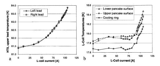
FIGURE 4. Temperature vs. current during first excitation of the L-coil to 105A. a) temperatures at upper ends of the HTS leads. b) temperatures at surface of L-coil pancakes and at the coil cooling ring.
