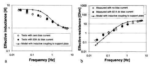
FIGURE 3. Results from the L-coil ac excitation experiments. a) Coil inductance vs. frequency. b) Effective coil resistance vs. frequency.
