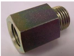
Male 9/16-18 Straight Thread O-Ring x Female 1/4" NPT
