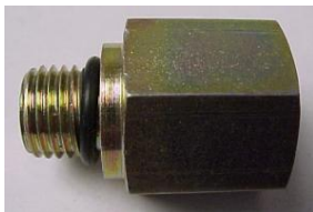
Male 7/16"-20 Straight Thread O-Ring x Female 1/4" NPT
