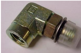
90 Elbow Male 9/16 – 18 Straight Thread O-Ring x Female 1/4" NPT
