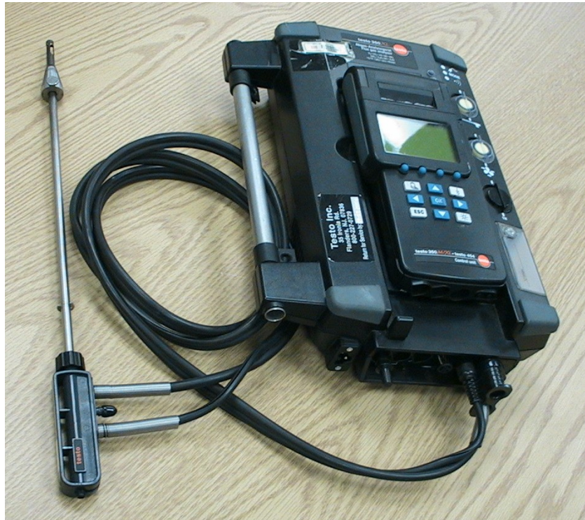
Figure 13 Testo 350XL Emissions analyzer system (O 2 , NO 2 , NO, SO 2 , CO, CO 2 )
