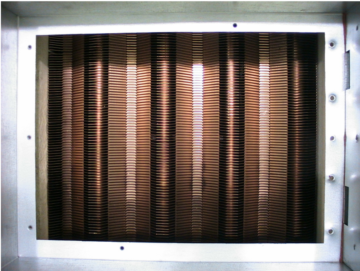
Figure 8 Tightly finned copper low mass heat exchanger of a gas-fired heater
