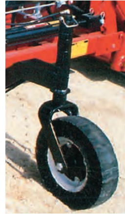
The optional, adjustable tailwheel provides extra support for the main beam — a real plus when working on rugged terrain.
