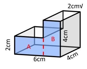
Volume= cross sectional area × lengthCross sectional area= area A + area B=  $(4 \times 2) + (2 \times 4)$ =  $8 \text{ cm}^2 + 8 \text{ cm}^2$ =  $16 \text{ cm}^2$ Volume= cross sectional area × length
