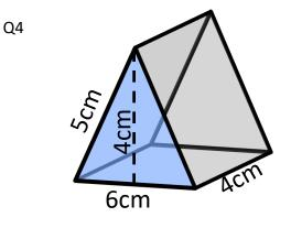
Volume = cross sectional area × length cross sectional area =  $\frac{1}{2}$  (base × height) =  $\frac{1}{2}$  (6 cm × 4 cm) = cm<sup>2</sup> Volume = cross sectional area × length = cm<sup>2</sup> × cm = cm<sup>3</sup>
