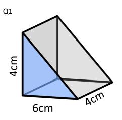
Volume = cross sectional area × length cross sectional area =  $\frac{1}{2}$  (base × height) =  $\frac{1}{2}$  (6 cm × 4 cm) = 12 cm<sup>2</sup> Volume = cross sectional area × length = 12 cm<sup>2</sup> × 4 cm = cm<sup>3</sup>
