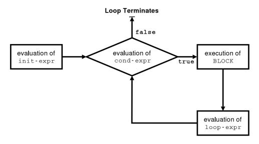
Figure 5.2: for-loop Flowchart
