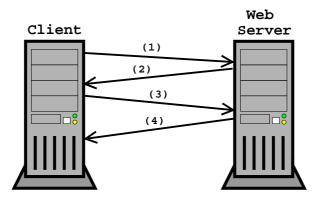
Figure 11.1: A simplified HTTP client-server interaction
