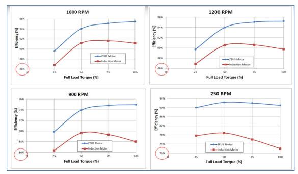
Fig. 6 Motor Efficiency, with VFD
