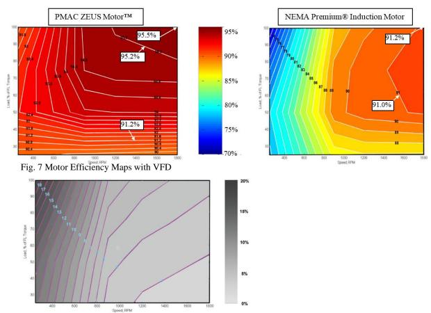
Fig. 8: Efficiency Advantage of PMAC ZEUS Motor<sup>TM</sup> over NEMA Premium Induction Motor
