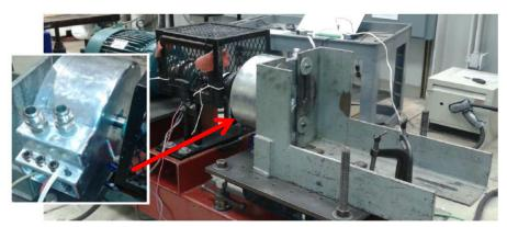
Fig. 5 ZEUS Motor<sup>TM</sup> under test; TENV cooling, liquid cooling
