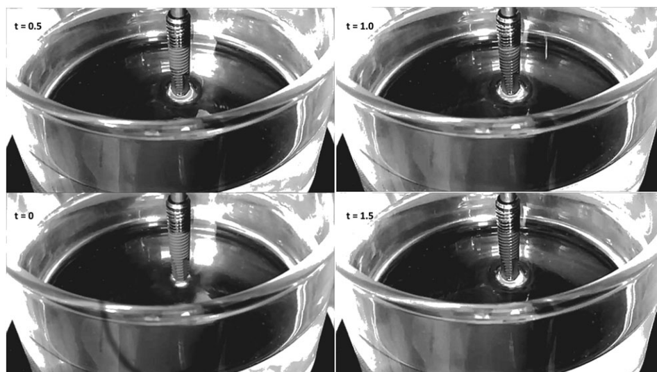
FIGURE 2 Timeframe image of the Wilhelmy plate experiment performed to evaluate capillary rise. Experimental time is reported in the frames
