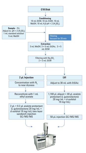
Figure.1 Flow diagram for pesticide extraction from water.
