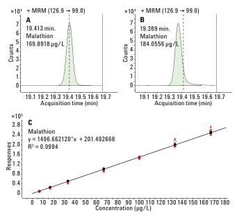
Figure 4. Malathion peak injected with (A) and without (B) analyte protectants. C) calibration curve of malathion using analyte protectant. The red triangles are injections without protectant.
