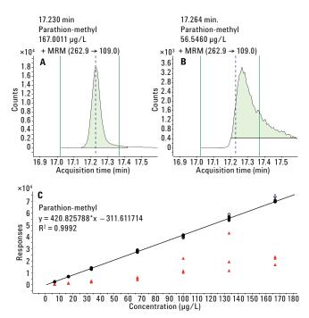
Figure 2. Parathion-methyl peak injected with (A) and without (B) analyte protectants, (C) calibration curve of
