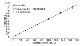
Figure 6. Calibration curve of vinclozolin performed by large volume injection with three replicated injections.
