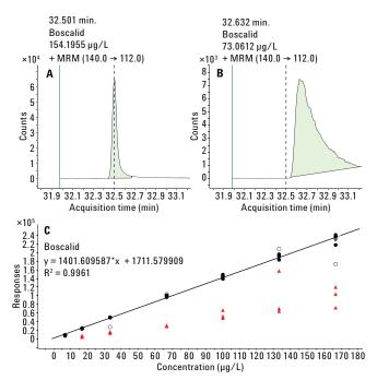
Figure 3. Boscalid peak injected with (A) and without (B) analyte protectants. C) Calibration curve of boscalid using analyte protectant. The red triangles are injections without protectant.
