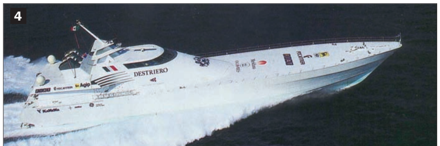
Two highly successful, and influential, large yachts—not designed by Peters—that meet the marine industry’s generally accepted definition of fast: the Mulder-designed 120’/36.6m Moonraker (top), and the Blount-designed 220’/67m Destriero . Moonraker ’s top speed is 67 knots; Destriero ’s, 60. For a detailed account of the latter’s design development, see Professional BoatBuilder No. 109, page 100.
