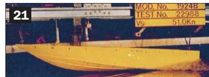
The towing-tank model, above , and lines plan, at left , for an even larger modified-V: a design proposal for a 128'/39m fast motoryacht for the German yard Abeking & Rasmussen. Weight summary and K-value on facing page.
