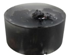
Sample impregnated with KEPT using KemVac
