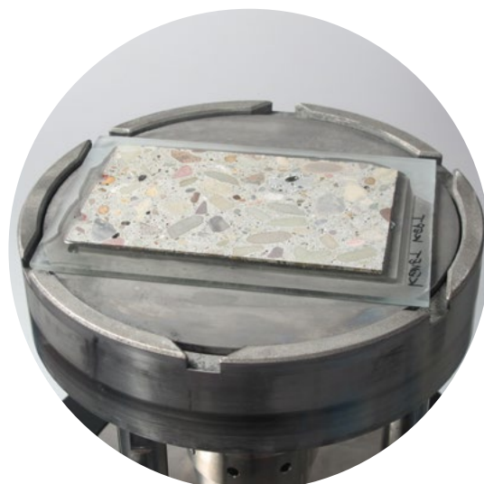
152 x 102 mm thin section of concrete
