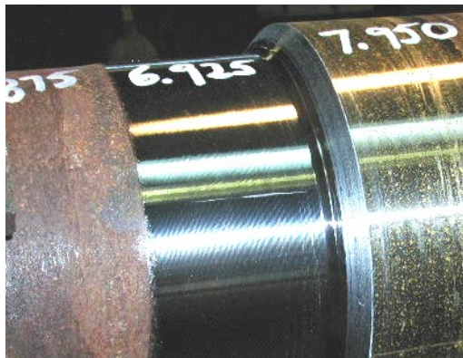
Figure 95 — Photo of machined area in way of old hard-banding removal showing longitudinal crack
