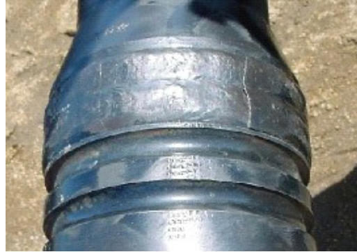
Figure 90 — Photo of new pin tool joint with longitudinal crack in hard-banding
