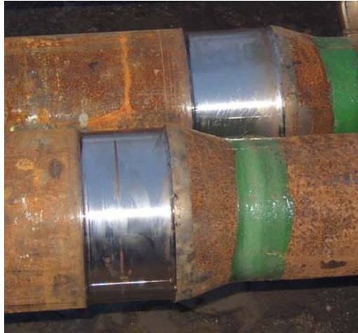
Figure 94 — Photo of box tool joints after removal of old hard-banding by machining
