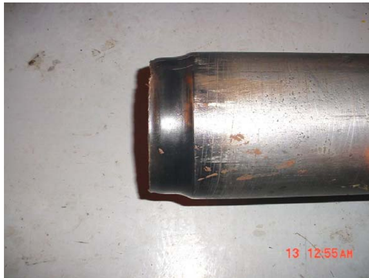
Figure 74 — Failure of Drill Pipe Body Rotated against Annular BOP Element
