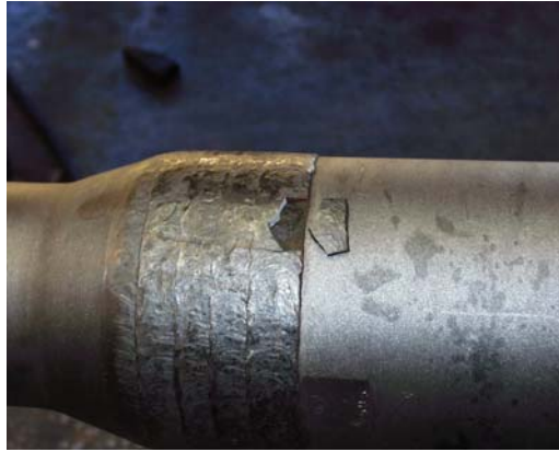
Figure 92 — Photo of new box tool joint with newly-applied hard-banding spalling-off
