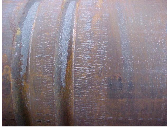
Figure 70 — Pin tool joint with heat checking revealed by dry magnetic particle inspection
