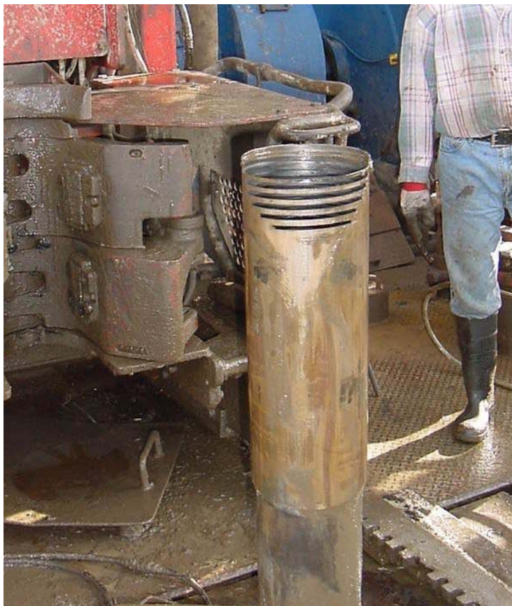
Figure 76 — Excessive wear to a box tool joint
