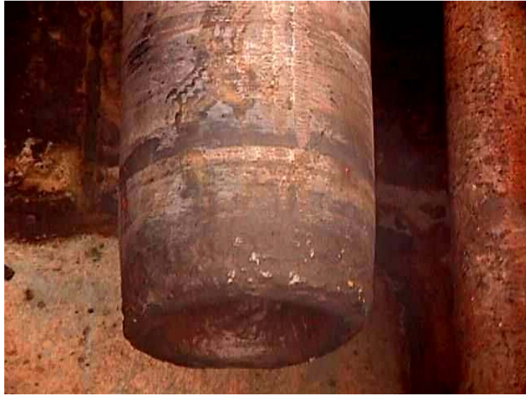
Figure 73 — Overheat pull failure of HWDP above the center wear pad
