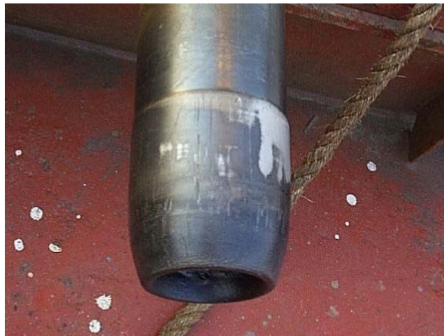
Figure 72 — Overheat pull failure of HWDP above the pin tool joint
