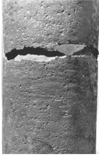
Figure D.46 — CO 2 corrosion on drill pipe OD
