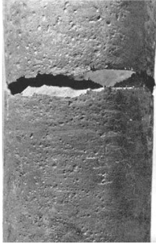
Figure C.46 — Figure 12 – CO 2 corrosion on drill pipe OD
