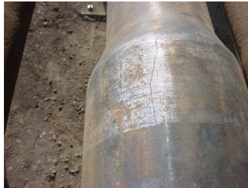
Figure 90 — Photo of new pin tool joint with longitudinal crack in hard-banding
