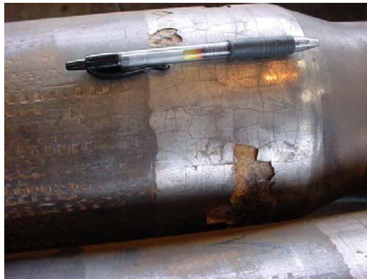
Figure 92 — Photo of new box tool joint with newly-applied hard-banding spalling-off
