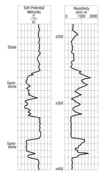
**Figure 1-2** Spontaneous potential and electrical resistivity logs identifying sandstones versus shales, and water-bearing versus hydrocarbon-bearing formations.
