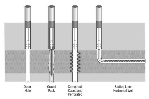
Figure 1-5 Options for well completions.
