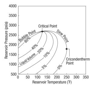
**Figure 1-3** Oilfield hydrocarbon phase diagram showing bubble-point and dew-point curves, lines of constant-phase distribution, region of retrograde condensation, and the critical and cricondentherm points.
