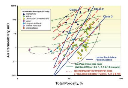
The image, drawn from Bust et al 2011, illustrates a wide range in permeability for any given value of porosity, which is a characteristic of complex pore geometry. Several different possible partitioning strategies are shown relative to the pore types; none captures pore type variation in this example completely and therefore the most fit-for-purpose schema in any given reservoir may vary from reservoir to reservoir.
