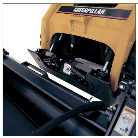
**Quick Coupler.** Work tools can be changed quickly and easily with the Cat Skid Steer's quick coupler system. The universal coupler interface features:
