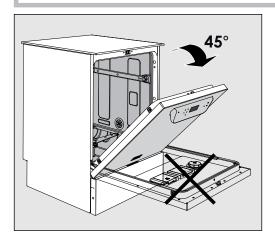
■ Open the door to an angle of approx. 45°. This ensures that the salt flows into the reservoir more easily.
