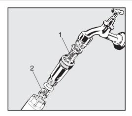
Install the filter (supplied in accessory pack) between the faucet valve and the inlet hose. The filter for DI water is made of chromium-nickel steel and can be recognized by its dull surface.
