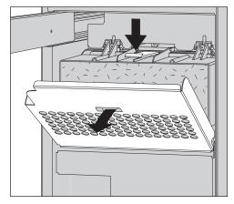
■ Release the filter grille and swing it downwards to open. The grille can also be removed completely.
