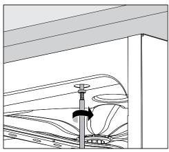
■ Screw the machine to the continuous worktop through the holes in the front trim on the left and right.
