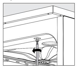
■ Remove the cover caps on the left and right and tighten the fixing screws. Then replace the cover caps.
