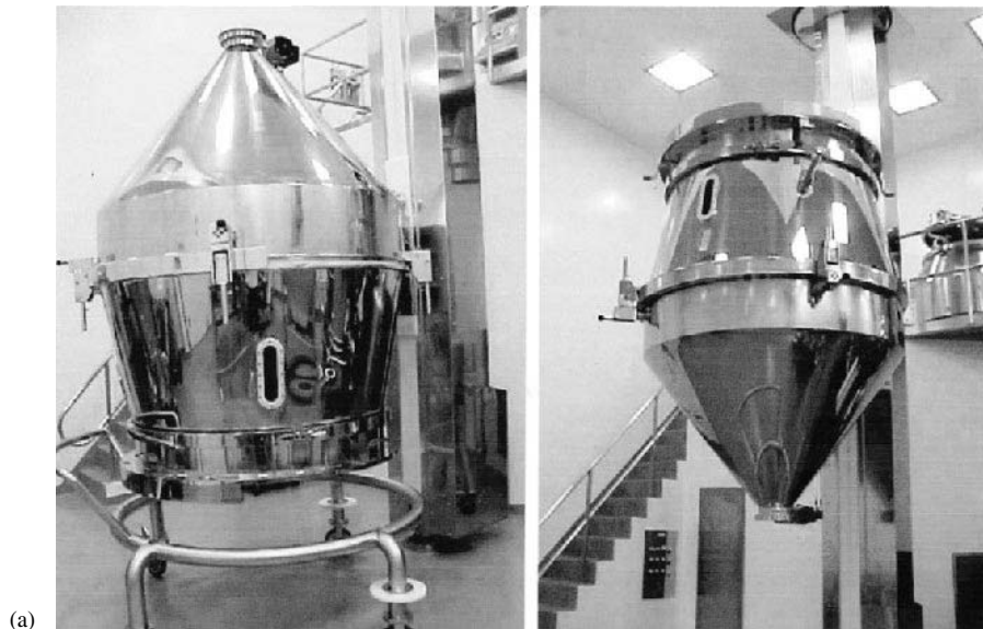
Figure 18 (a) Product discharge with a bowl dumping device. ( continues )
