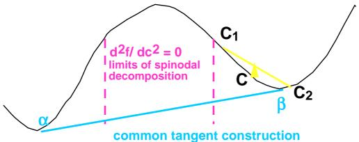
Net increase in F as compositions diverge – hence nucleation barrier, even though ultimately end up with overall lowering of energy when split into phases  $\alpha$  and  $\beta$ .
