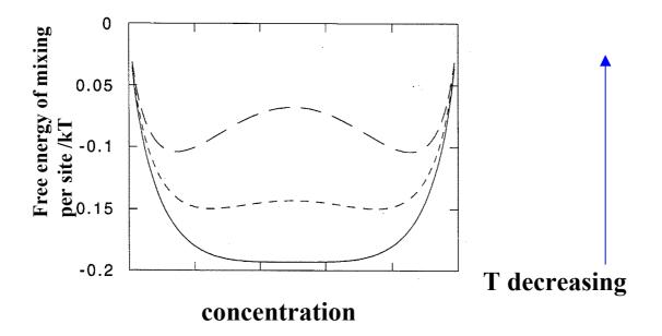
Knowing the form of the free energy curves as a function of T means that we can map out the limits of solubility etc.
