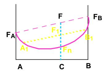
This can be lowered by going to compositions  $A_1, B_1$  to give free energy  $F_1$  etc
