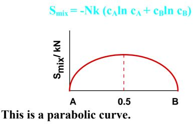
There is always a positive entropy gain on mixing (note the logarithms are negative) – so that entropic considerations alone will lead to a homogeneous mixture.
