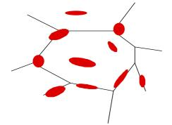
Large, well-separated precipitates, typically at grain boundaries, which do not provide much barrier to dislocation motion
