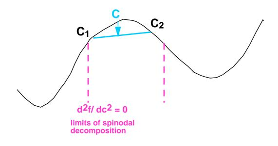
Start at composition c, split into 2 slightly different compositions  $c_1$  and  $c_2$  to give net lowering of energy.
