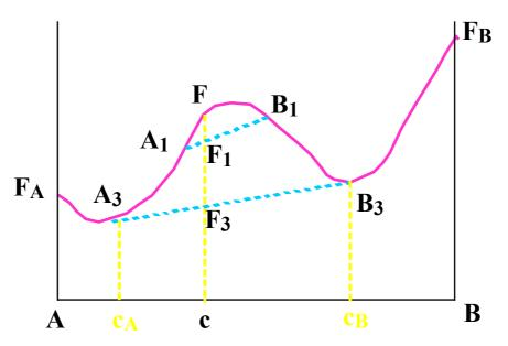
This can split into A<sub>1</sub> and B<sub>1</sub>; energy drops to F<sub>1</sub>.
