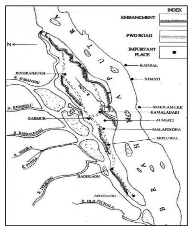
Figure 8-1: Embankment System of Majuli
