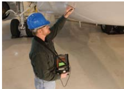
On-wing, wide-area scanning with arrays ensure complete inspection coverage of aluminum and composite structures.
