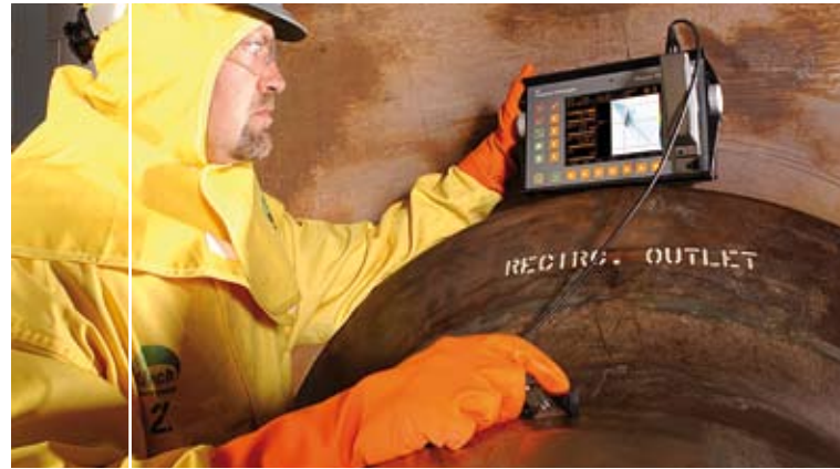
The portable, rugged and battery-operated Phasor XS is designed to be used in the most demanding circumstances including bagging for nuclear anti-contamination.
