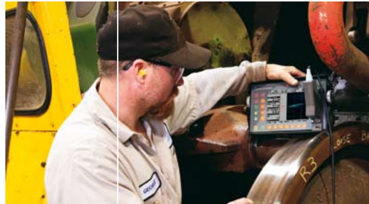
Specially designed transducers allow wheel inspections to be carried out faster, still providing more reliable results.
